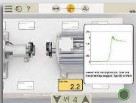
Soft Foot check on both machines
